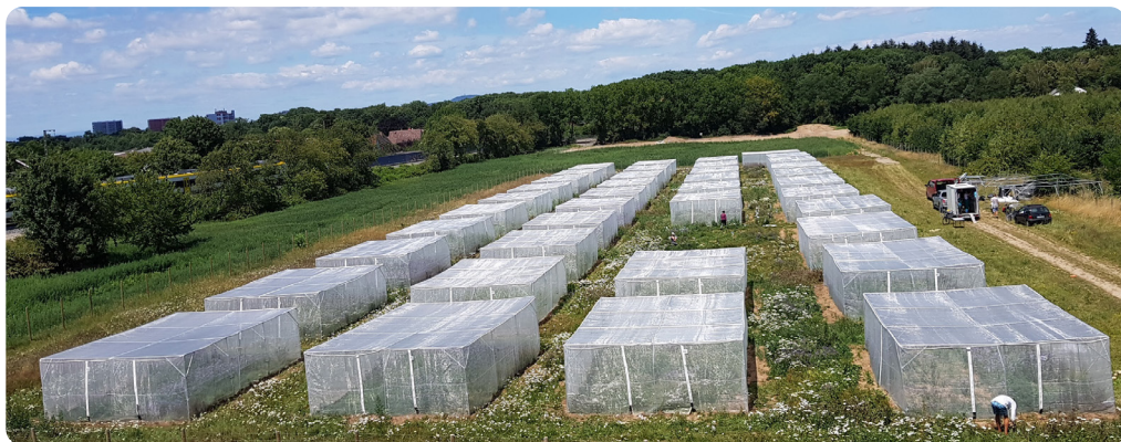
Figure 1: Semi-field experiments consist of large flight cages that enclose bees with flowering resources that are either pesticide-treated or not. This allows for assessing (interactive) effects of flowering resources and pesticides applied according to label guidelines.
